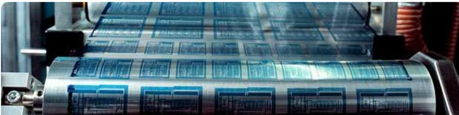
Figure 14 Printed RFID's that are large area devices that include both ariel and logic<sup>33</sup>.
